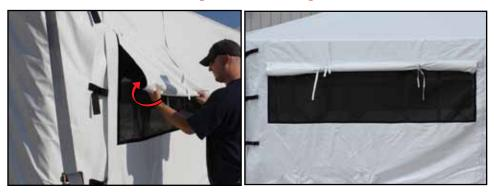
27. To roll up the door stand inside the tent, tightly roll up on top of the door. Tie off with tie tie
