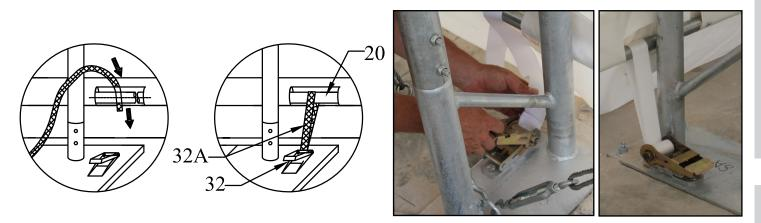
17. Tension the cover on the frame from side to side, taking up the slack in the tie bands by ratcheting the mechanisms, tightening cover. Evenly adjust ratchets on both sides of the roof to take out the wrinkles. DO NOT FULLY TIGHTEN YET. Leave adequate slack so that the cover can also be adjusted front to back in the next step.
