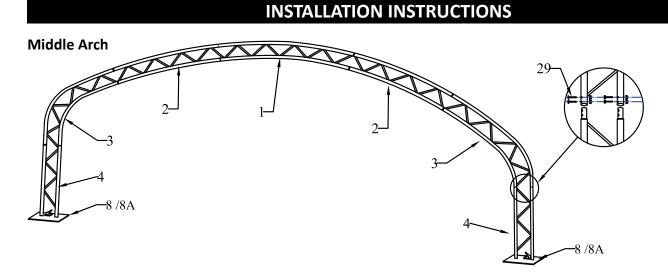
4. Erecting the arches: Erect the front arch by using ropes. Tie and secure the rope to a heavy object to secure the arch standing temporarily. Lift the arch and secure the base flanges.
