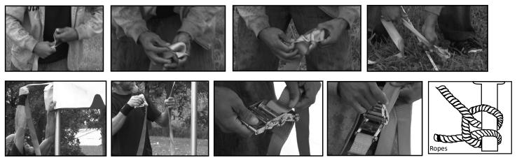
17. Roll excess ratchet straps and secure into the ratchet buckle.
