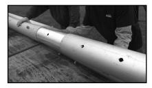
9. Insert the center pole pin through the center nipple/floor flange assembly; make sure that the pin is not caught on any part of the tent top. Lift the top using the center pole and set pole at an angled position so the top is completely off the ground. Insert a tent stake into the helper hole on the center pole if available.
