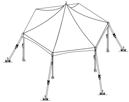
17. Make sure the legs are straight then secure each base plate by driving a 24" anchoring hooks into the smaller hole of the base plate tighten all ratchet assemblies.
