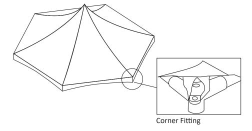
9. Fasten the loop end of the 8' loop strap (B) to the carabiner. Secure the carabiner to the hook on the outside of the corner fittings (the same hook that the tent top is secured to).
