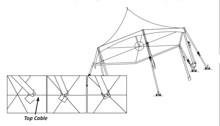
16. Install the remaining two legs (8') and ratchet assemblies; be sure the smaller holes of the base plate are facing the interior of the tent.
