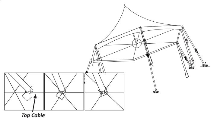
15. Install the remaining two legs (8') and ratchet assemblies; be sure the smaller holes of the base plate are facing the interior of the tent.
