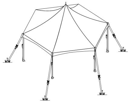
16. Make sure the legs are straight then secure each base plate by driving a 24" anchoring hooks into the smaller hole of the base plate tighten all ratchet assemblies.
