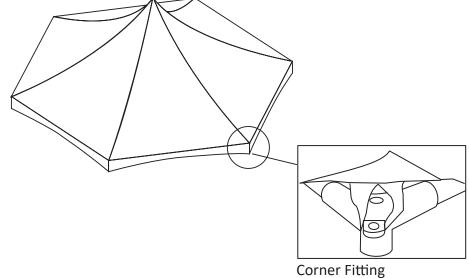
8. Fasten the loop end of the 8' loop strap (B) to the carabiner. Secure the carabiner to the hook on the outside of the corner fittings (the same hook that the tent top is secured to).
