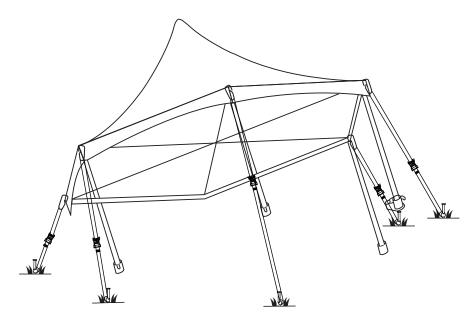
12. Fasten the 6' series loop strap (D) to each corner through the two metal O rings on the tent top, then through the end loop and tighten.
