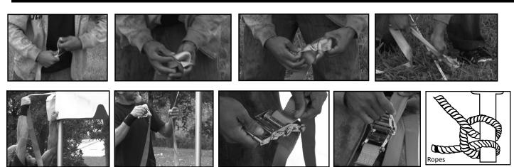
19. Roll excess ratchet straps and secure into the ratchet buckle.
