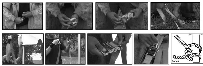
17. Roll excess ratchet straps and secure into the ratchet buckle.
