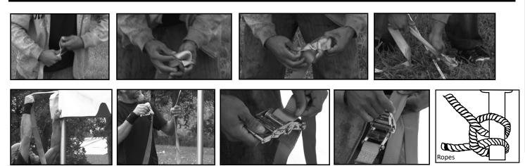
16. Roll excess ratchet straps and secure into the ratchet buckle.
