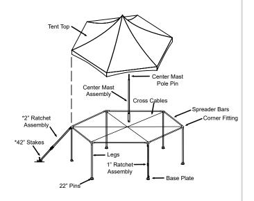
General frame construction shown on a 20' Hex \*2" ratchet assembly and 42" stakes are installed at all corner locations.
