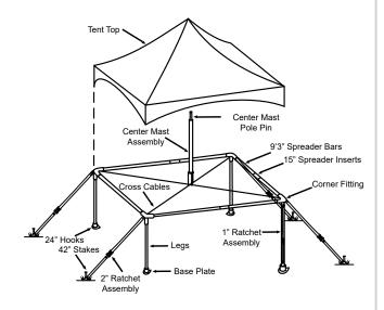
General frame construction shown on a 20' x 20'
