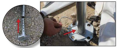
9. Lift one side of the frame up and slide the legs (Green/HT2GST80) with base plates into the bottom of the two corner fittings (F01CORHT) and pin using pin and bail (HT570). Slide the pin through the hole in the corner fitting and leg hole then connect the bail end around the pin.
