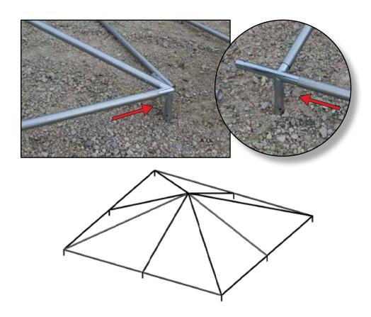
7. Pull the tent top over the frame. IMPORTANT: Leave the sidewalls on top of the frame.
