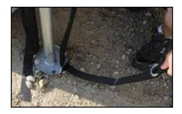
22. Tighten each strap by running the tail end of the strap through both D rings and then back through the lower D ring. Pull the tail end downward to tighten. Use a foot if necessary to tighten the straps.
