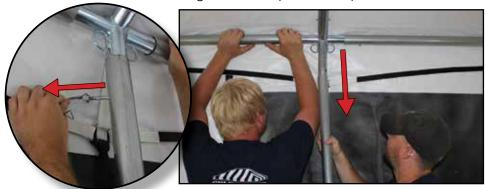
On one side remove both legs with base plates from the corners, place off to the side, and carefully set the frame down.
