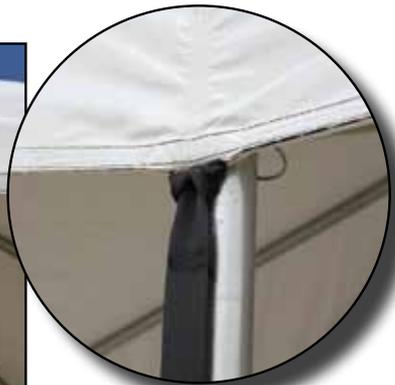
13. Locate the remaining tent top straps, 120" (300 cm) in length, and attach. Attach the loop end through the 1½" (3.81 cm) welded D ring, run the rest of the strap through the loop and outside slot of the base plate, and pull tight.
