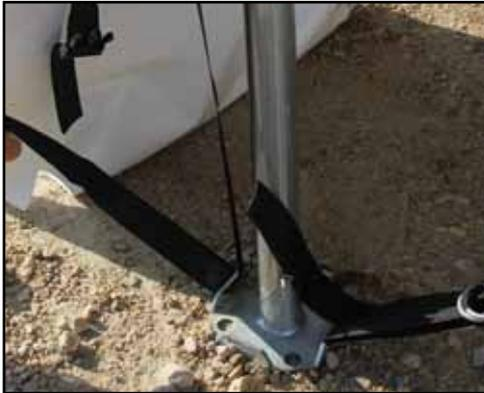
18. **NOTE:** *Center tent top before tightening all straps by centering the patch with the 8 way crown.* Tighten each strap by running the tail end of the strap through both D rings and then back through the lower D ring. Pull the tail end downward to tighten. Use a foot if necessary to tighten the straps.
