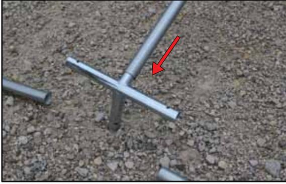
6. Connect each of the 88" (223.52 cm) spreader poles (Red/HT2GST88) between each corner (F01CORHT) and each side tee fittings (F02STHT) all the way around the perimeter of the frame. Lining up the holes until the push pins engage.
