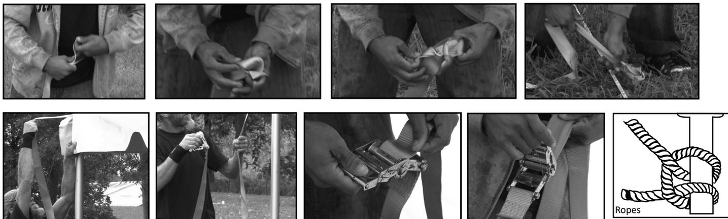
18. Roll excess ratchet straps and secure into the ratchet buckle.
