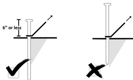
Stakes driven vertically have a greater holding strength than stakes driven at an angle. Vertically is defined as straight up down or angled up to 10° away from the tent, canopy, structure, or shelter.
