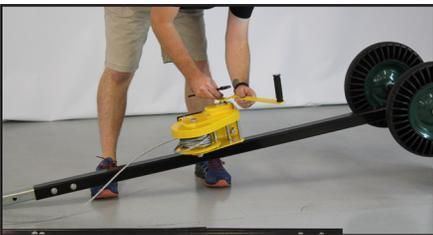
4. Unroll the winch cable so that there is enough slack to move the upper beam above the jack frame piece.
