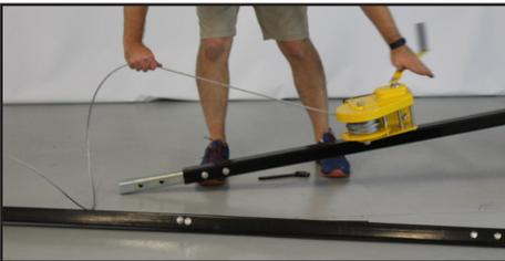
5. Align the upper beam with the jack frame piece; make sure that the cable is not twisted around the beams. If the jack is being assembled with the base plate downward, the kickstand will be on the right side of the beam looking from the wheels. Make sure the cable runs straight from the winch to the pulley at the top of the upper beam.
