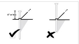
Stakes driven vertically have a greater holding strength than stakes driven at an angle. Vertically is defined as straight up down or angled up to 10° away from the tent, canopy, structure, or shelter.
