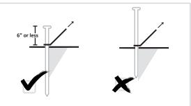
Stakes driven vertically have a greater holding strength than stakes driven at an angle. Vertically is defined as straight up down or angled up to 10° away from the tent, canopy, structure, or shelter.
