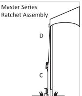
A. Ratchet Buckle with Loop Strap B. Loop Strap C. Master Series Ratchet Buckles Loop Strap w/ O Ring
