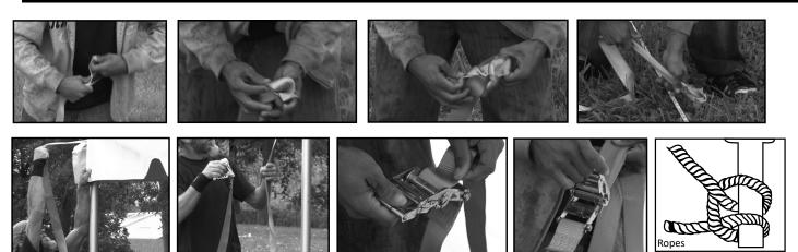
20. Roll excess ratchet straps and secure into the ratchet buckle.
