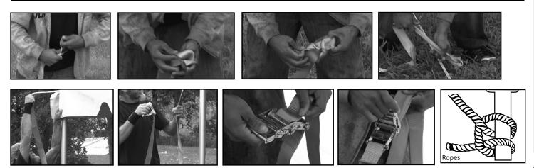
18. Roll excess ratchet straps and secure into the ratchet buckle.
