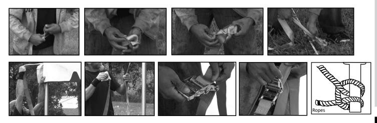
16. Roll excess ratchet straps and secure into the ratchet buckle.
